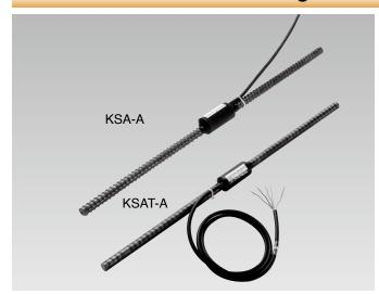
The KSA-A and KSAT-A are used to measure stress applied to structural reinforcing bars, and are normally welded at both ends to form part of the reinforcement arrangement. And the meters are with built-in temperature sensor, making possible simultaneous measurement of stress and temperature. The KSA-A has strain gauge type temperature sensor, while the KSAT-A has a thermocouple that can be used to measure actual temperature.
