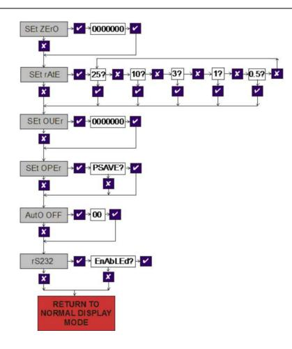
A Calibration Menu, which is used to calibrate each of the two ranges with independent scales, as well as setting the display resolution for each range.
