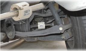
Frictional Torque Sensor FGDH
