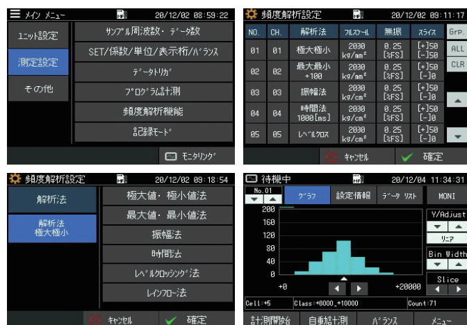
Frequency measurement setting screen and graph display screen using TMR-381 display unit
