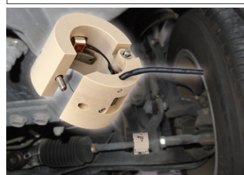
Installation on steering tie-rod of a car
