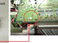
Lead wire out wiring example Taking out from screw end
