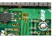
When electronic components are mounted on a board, mounting pressure is applied and some strain is generated in the board. Furthermore, the strain is generated when dividing the board as well. Investigation of what type of strain is generated through the measurement of strain.
