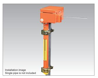
The NKLG-AB ground extension gauge is used to measure the displacement of a ground surface. A super-invar wire is set
