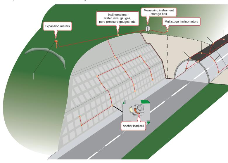
TML-NET is our original network that enables measurement control and data transfer via a 2-wire network line and also provides power supply.
