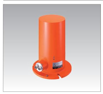
The NKLA-A is also for the same measurement while it can be used with the network measurement system TML-NET. Special anchors are mounted at specified positions inside a borehole and the amount of positional displacement between each anchor and the ground surface level is measured. Anchors can be mounted at the maximum of six levels inside one borehole.
