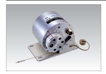
The NKLG-BB ground extension gauge is placed near the ground surface to measure the displacement of a ground slide. A super-Invar wire is set between a stanchion at a reference point (fixed stanchion) and a stanchion at a measurement position (mobile stanchion) and this gauge is mounted on the stanchion at the reference point. The waterproof and environmental resistance features make this gauge suitable for on-site
