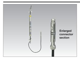
This is the inclinometer developed to automatically measure the displacement of the ground or structure.
