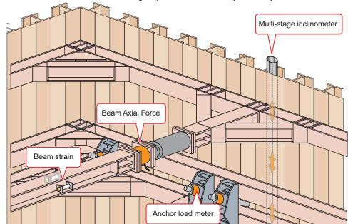
Comparison of multi-stage inclinometer measurement systems by TML-NET
