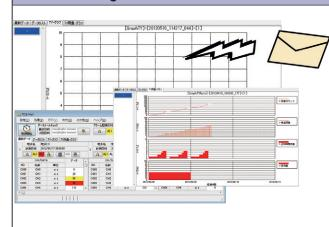
Measurement data from interval timers and other devices using our data loggers are sent via e-mail using a data mail converter.
