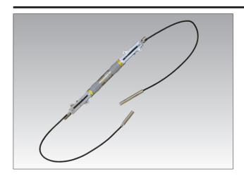
An inclinometer developed to automatically measure the displacement of ground and structures
