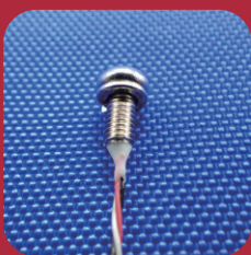
M3 axial force bolt installation example
