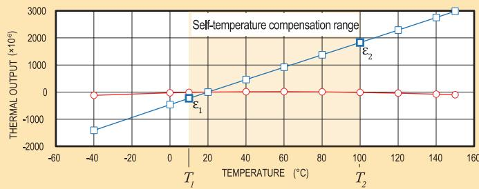
Linear expansion coefficient of certain materials in the self-temperature compensation range ( $10-100^\circ\text{C}$ ).
