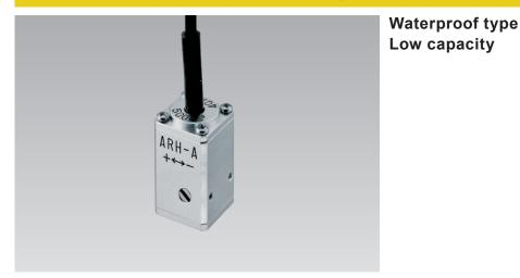
The ARH-A acceleration transducer has a waterproof structure. It is installed in water or ground or embedded in concrete. The rigid waterproof structure makes this transducer suitable for use in an adverse environment or for outdoor use. Protection ratings: IP67 equivalent
