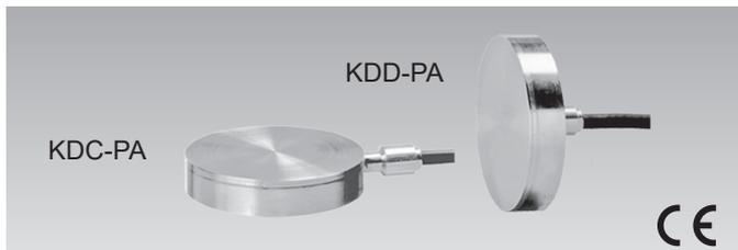
The KDC-PA and KDD-PA are anticorrosion stainless-steel soil pressure gauges each 100 mm in outside diameter. They are used to measure the pressure in soil in ocean or coastal civil engineering structures and to measure the dynamic pressure of waves. The difference between these two models is the way the cable is attached to the gauge body.
