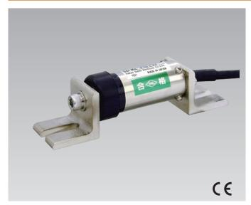
The KG-A crack displacement transducer is set across a crack on the surface of concrete or across a joint between two concrete layers to measure the displacement of openings. The waterproof feature allows this transducer to make accurate and stable measurement outdoors over a long period of time. It is mounted using an anchor bolt (KGF-11) or a mounting metal piece (KGF-31).
