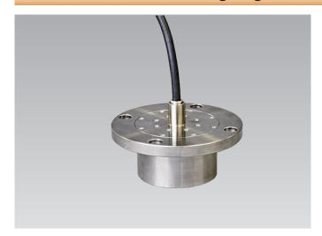
The KKB-PA is a transducer to measure the subgrade reaction force (bearing force) acting on the caisson cutting edge. The transducer is installed so that the sensing surface of the transducer is positioned in the same surface with the bottom surface of the caisson cutting edge. The subgrade reaction force is measured during the immersion and settlement of the caisson.
