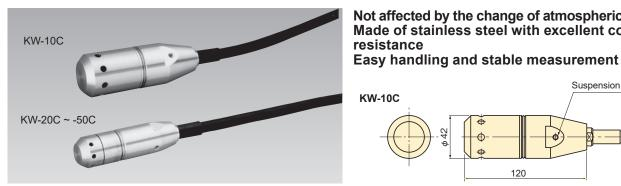
The KW-C is a hydraulic water level transducer that measures the level of water in dams and rivers and the level of under-ground water in ground in landslide areas. Effects of changes in atmospheric pressure do not need to be compensated, so highaccuracy measurement can be made. Protection ratings: IP68 equivalent
