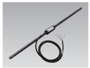
The KSAT-A are used to measure stress applied to structural reinforcing bars, and are normally welded at both ends to form part of the reinforcement arrangement. And the meters are with built-in temperature sensor, making possible simultaneous measurement of stress and temperature. The KSAT-A has a thermocouple that can be used to measure actual temperature.
